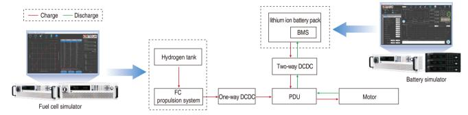
Compared with the traditional diesel engine as the motive power, the fuel cell power propulsion system has the advantages of no pollution, no emission and low noise. It is very suitable for applications requiring long driving mileage and high stability.
