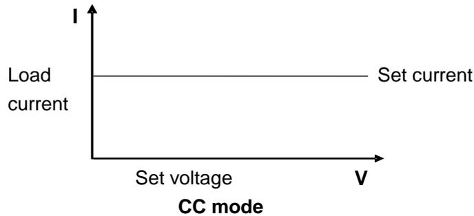
Fig. 3-1 Voltage-Current Relation Schema under CC Mode
