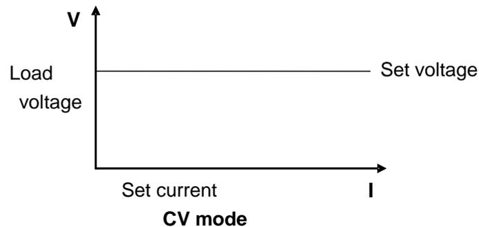
Fig. 3-2 Voltage-Current Relation Schema under CV Mode
