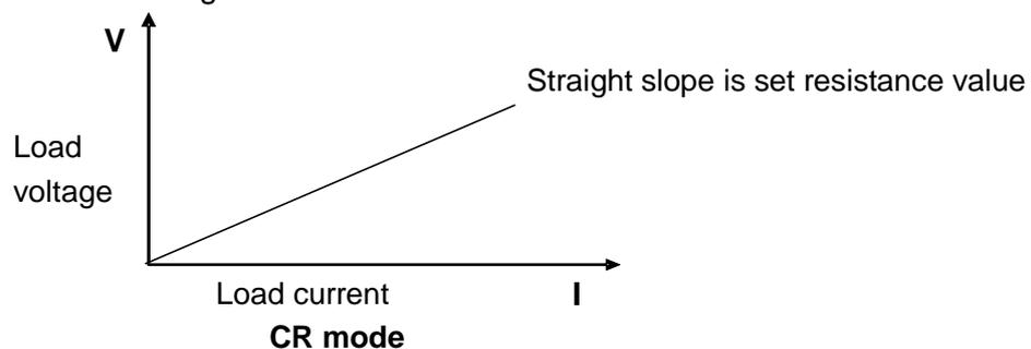
Fig. 3-3 Voltage-Current Relation Schema under CR Mode
