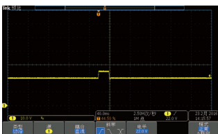
D/D Converter Surge Testing
