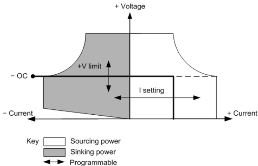
The heavy solid line illustrates the locus of possible operating points as a function of output. As shown by the vertical portion of the line, the output current remains regulated at its programmed setting as long as the output voltage remains within its limit setting. A CC (constant current) status flag indicates that the output current is being regulated and the output voltage is within its limit settings.
