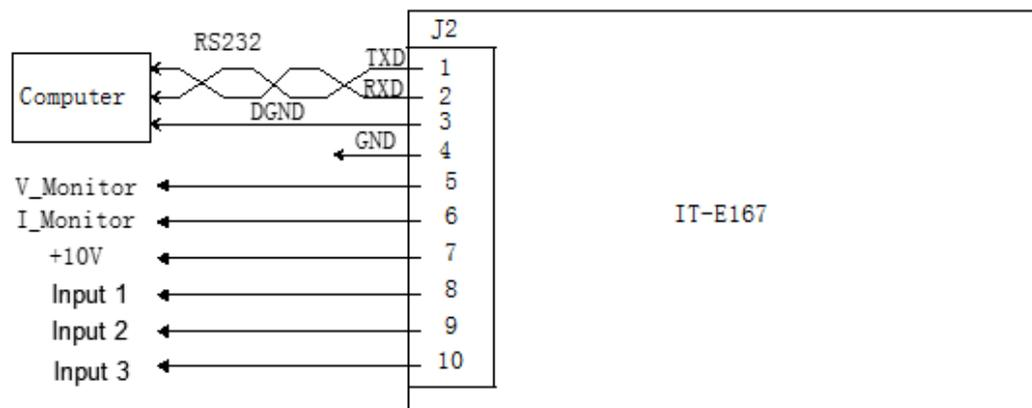
When using the RS-232 interface for communication, connect the pin 1, pin 2, and pin 3 of the IT-E167 to the PC. The pin description is as follows:
