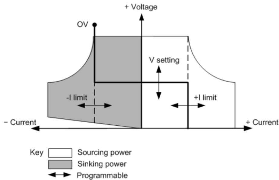
The heavy solid line illustrates the locus of possible operating points as a function of output. As shown by the horizontal portion of the line, the output voltage remains regulated at its programmed setting as long as the load current remains within the positive or negative current limit setting. A CV status flag indicates that the output voltage is being regulated and the output current is within its limit settings.
