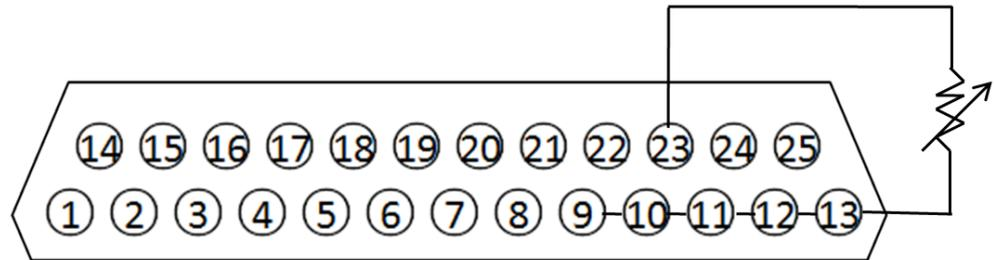
To set the 0~5V/0~10V or 0~5K $\Omega$ /0~10K $\Omega$  external analog setting range, the operations as follows:
