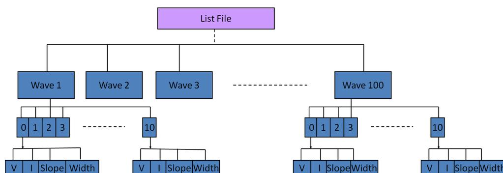
List file can select any one from 100 waves. Each List file can select 10 wave files at most and combine them into a List file based on sequence.
