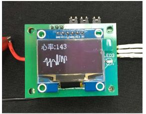
DUT: a heart rate tester module
