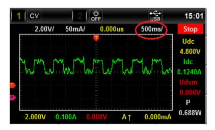
The overall waveform under 500ms/div setting
