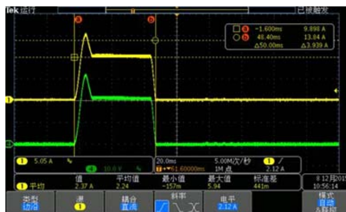
Figure2. LED lamp test result which is tested by a traditional power supply
