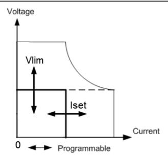
The heavy solid line illustrates the locus of possible operating points as a function of output. As shown by the vertical portion of the line, the output current remains regulated at its programmed setting as long as the output voltage remains within its limit setting. A CC (constant current) status flag indicates that the output current is being regulated and the output voltage is within its limit settings.
