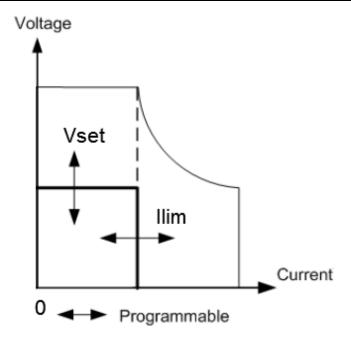
The heavy solid line illustrates the locus of possible operating points as a function of output. As shown by the horizontal portion of the line, the output voltage remains regulated at its programmed setting as long as the load current remains within the current limit setting. A CV status flag indicates that the output voltage is being regulated and the output current is within its limit settings.
