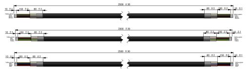
The yellow-green wire is grounding wire, which is connected to the PE terminal of power input on the rear panel; the others are live wires, which are correspondingly connected to the L1, L2 and L3 terminals of power input on the rear panel of the instrument.
