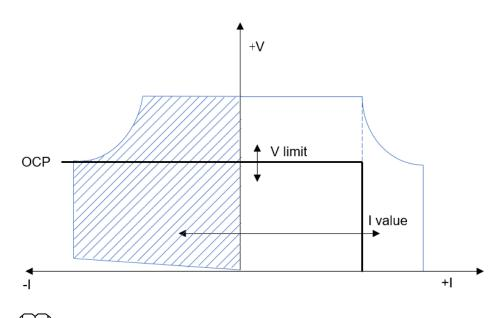
In sink mode, there is a minimum operating voltage. The minimum operating voltage specification data corresponding to different voltage models are as follows.
