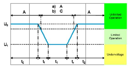
FTest pulse parameters for E48-10 Starting pulses
