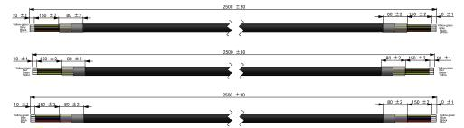
The yellow-green wire is grounding wire, which is connected to the PE terminal of power input on the rear panel; the others are live wires, which are
