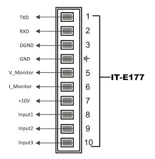
When using the RS-232 interface for communication, connect the pin 1, pin 2, and pin 3 of the IT-E177 to the PC. The pin description is as follows:
