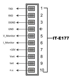
When using the RS232 interface for communication, connect the pin 1, pin 2, and pin 3 of the IT-E177 to the PC. The pin description is as follows:
