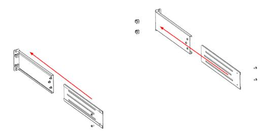
6. Fasten the hexagonal socket head combination screws M4x8 (6pcs) to the rear mounting lug connections already installed on the cabinet and already installed on the rear of the instrument as shown by the red arrows in the figure below.
