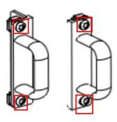
Fasten the hexagonal socket head combination screws M4x8 (6pcs) as shown by the red arrows in the figure below to the rear mounting lug connections already installed on the cabinet and already installed on the rear of the instrument.
