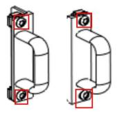
6. Fasten the hexagonal socket head combination screws M4x8 (6pcs) as shown by the red arrows in the figure below to the rear mounting lug connections already installed on the cabinet and already installed on the rear of the instrument.
