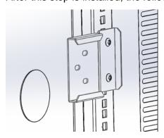
5. Drop the instrument with the carrying handle and rear connector installed into the cabinet and fasten the cassette nut combination (4pcs) to the front mounting ears of the instrument and the cabinet.
