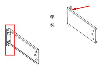
4. Drop the instrument with the carrying handle and rear end connector installed into the cabinet and fasten the cassette nut combination (4pcs) to the front mounting ears of the instrument and the cabinet.
