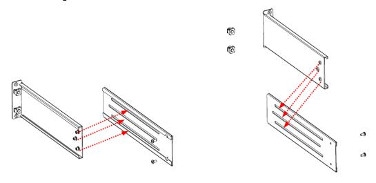
After the installation is completed, the side is shown below (shortest and longest).
