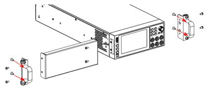
2. Install the cross small pan head screws M4x8 (12pcs) in the IT-E158C kit to both sides of the instrument as shown by the red arrows in the figure below.
