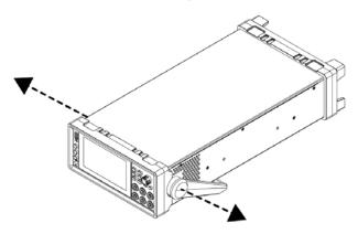
2. Refer to the figure below and turn the handle from position A to B. When turning the handle, take care to place the instrument gently to prevent it from falling.
