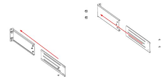
7. Fasten the hexagonal socket head combination screws M4x8 (6pcs) to the rear mounting lug connections already installed on the cabinet and already installed on the rear of the instrument as shown by the red arrows in the figure below.
