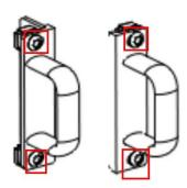
6. Adjust the length of the retractable kit according to the depth of your cabinet.
