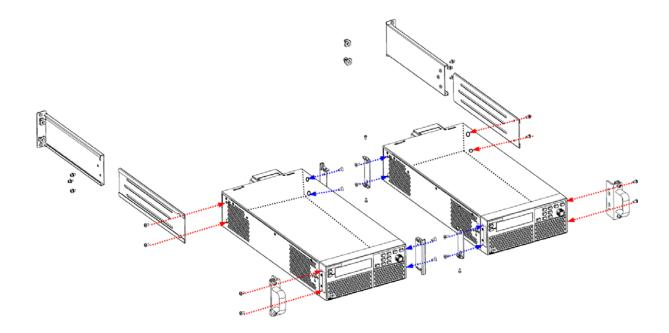
3. According to the red arrow shown in the figure below, first merge the connection pieces in the middle of the two instruments (at note A in the figure), and after aligning the mounting holes in the middle, fasten them (at note B in the figure) with cross small pan head screws M3x6 (4pcs).
