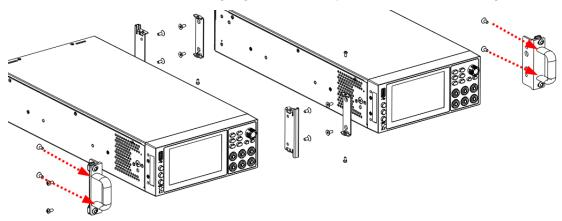
2. Install the cross small pan head screws M4x8 (8pcs, shown by red arrows) and cross countersunk head screws M4x10 (8pcs, shown by blue arrows) to both sides of the instrument as shown by the arrows in the figure below.
