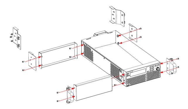
3. Fasten the cassette nut combination (4pcs) in the IT-E158C kit to the rear mounting lug connector (2pcs) and the square hole strip in the middle of the side of the ITECH cabinet as shown by the red arrow in the figure below.
