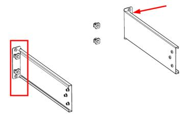
5. Drop the instrument with the carrying handle and rear end connector installed into the cabinet and fasten the cassette nut combination (4pcs) to the front mounting ears of the instrument and the cabinet.
