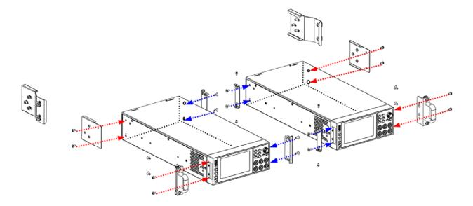
3. According to the red arrow shown in the figure below, first merge the connection pieces in the middle of the two instruments (at note A in the figure), and after aligning the mounting holes in the middle, fasten them (at note B in the figure) with cross small pan head screws M3x6 (4pcs).
