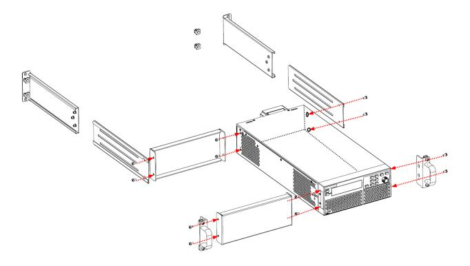
3. Fasten the cassette nut assembly (4pcs) to the rear mounting lug connectors (2pcs) and the square hole strip on the side of the cabinet as shown by the red arrow in the figure below.
